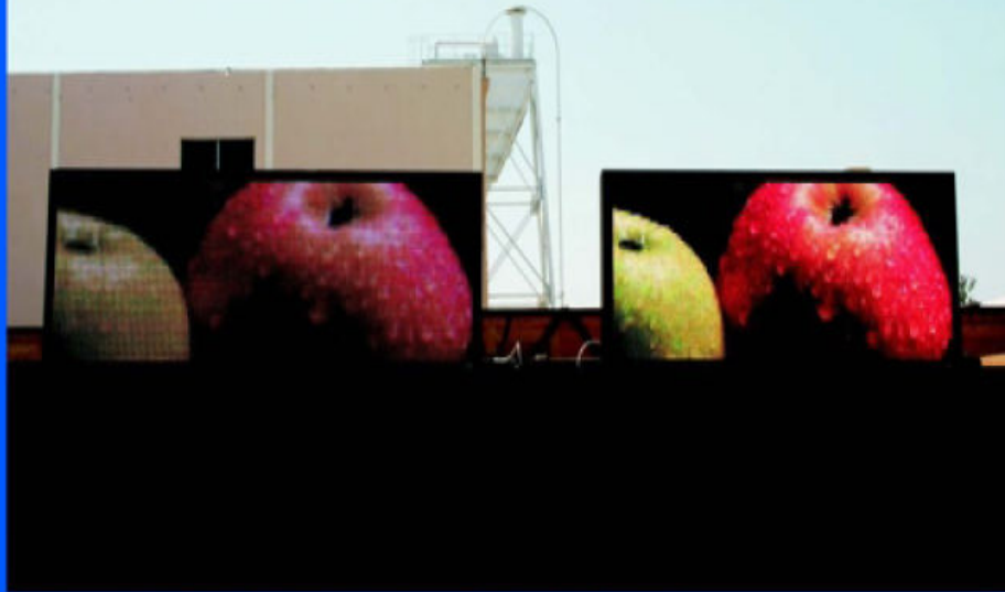
Left: 20mm video display with 3 LED per pixel (matrix: 48x128) Right: 20mm video display with 5 LED per pixel (matrix: 48x96) LED Spec: Same model Nichia Super Ovals Environment: 90 F, bright California summer, 11:30am, 6/25, 2006
